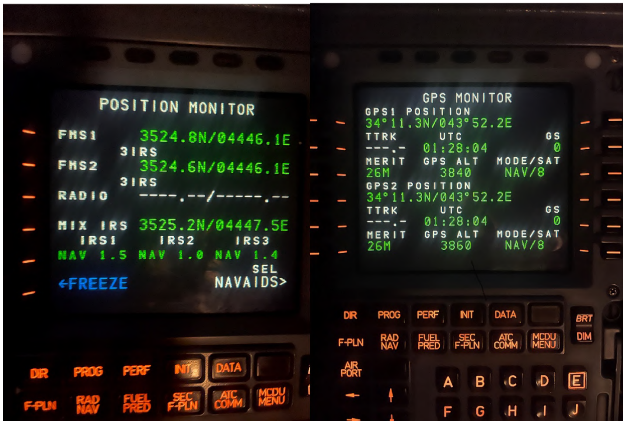
An example of GPS Spoofing in action during cruise phase: FMS position shows correct, GPS is being spoofed. Note also GPS Altitude incorrect, True track (TTRK) and Ground Speed (GS) values are zero - all indications of spoofing. A320, ORBB FIR.
