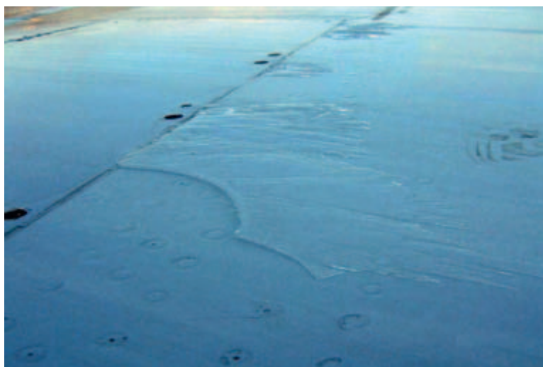
Figure 2 Clear-ice contamination on the wing
