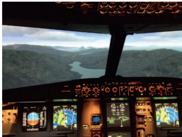
Figure 5 Vágar simulator scenery. The RNP AR training was given in a full flight simulator with very detailed scenery of Vágar.
