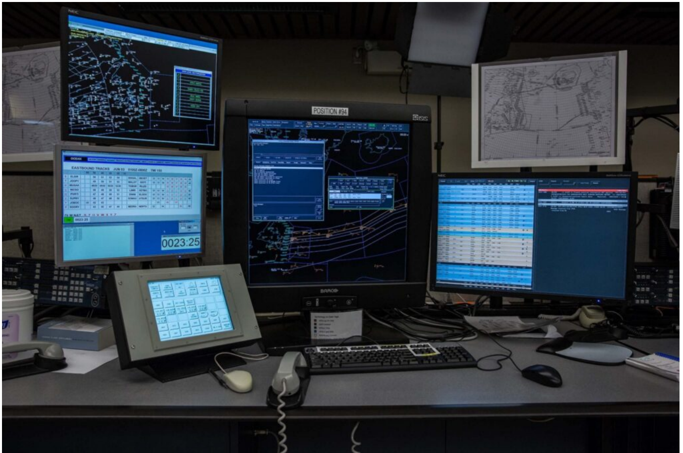
ATC NAT Controller station
