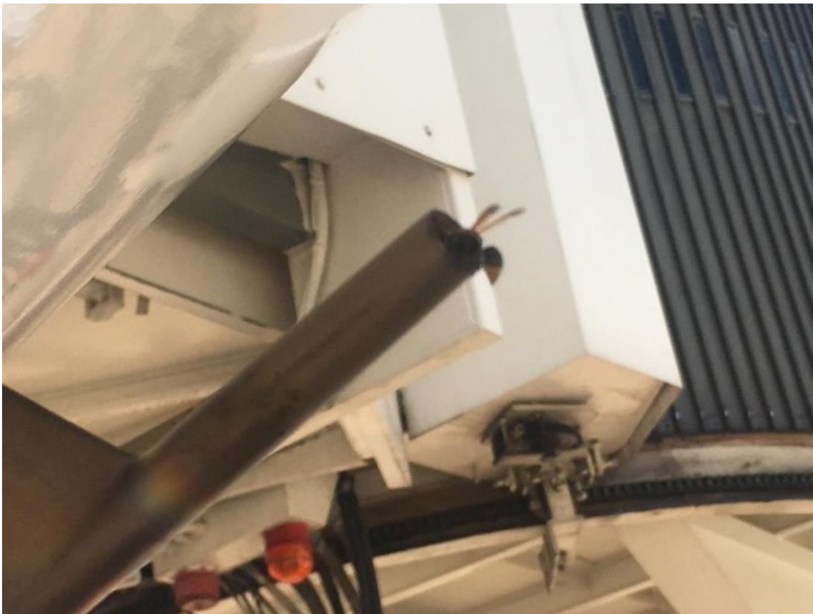
A Mud Dauber Wasp entering the pitot tube of a 737.
