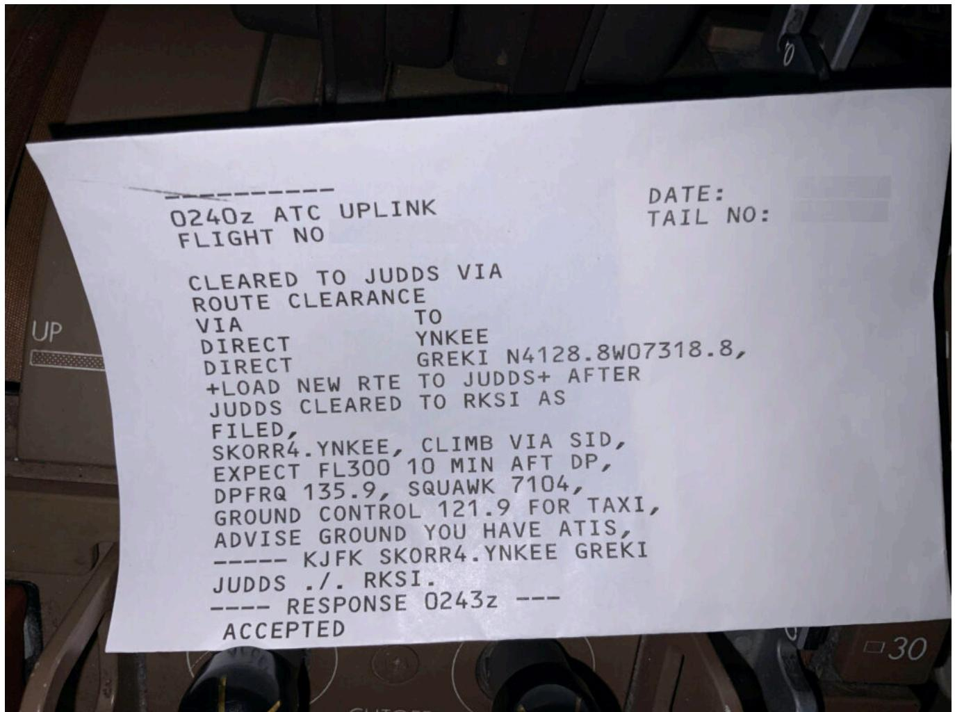
Unfortunately, in this instance the crew **mis-interpreted their clearance as direct to the waypoint YNKEE**. This was further compounded by the issue above – when the new route was loaded, **their SID was dropped from the flight plan**.
