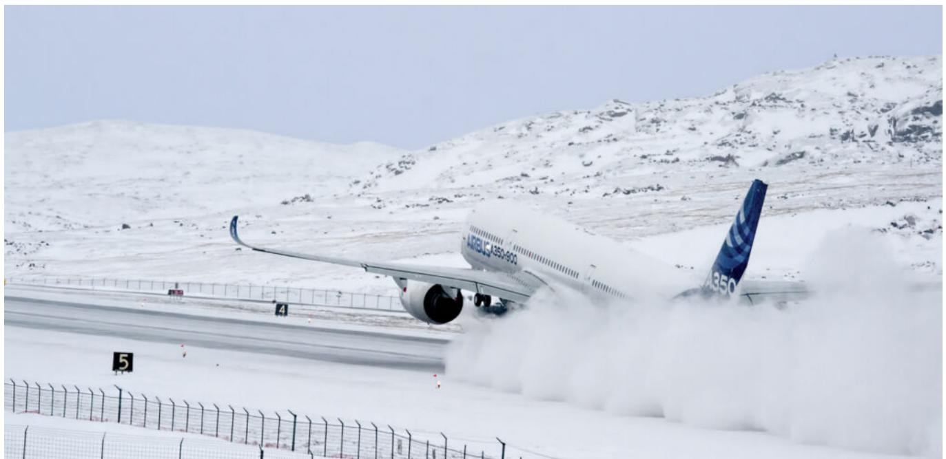
A350 contaminated runway tests (credit: Airbus).
