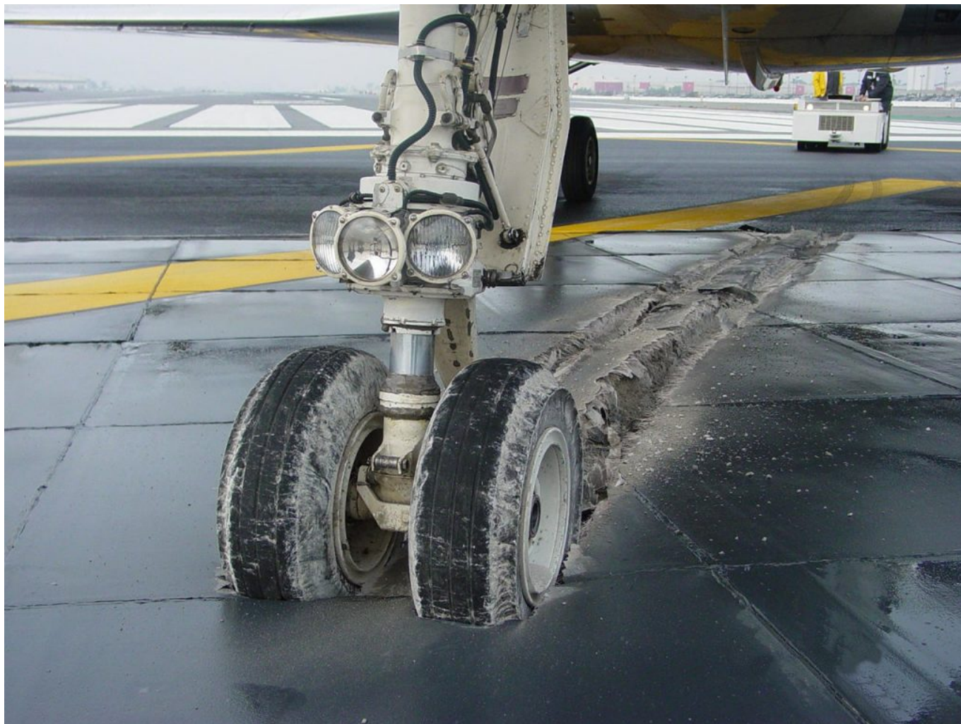
EMAS Arrestor Pad in action. Courtesy: Runway Safe
