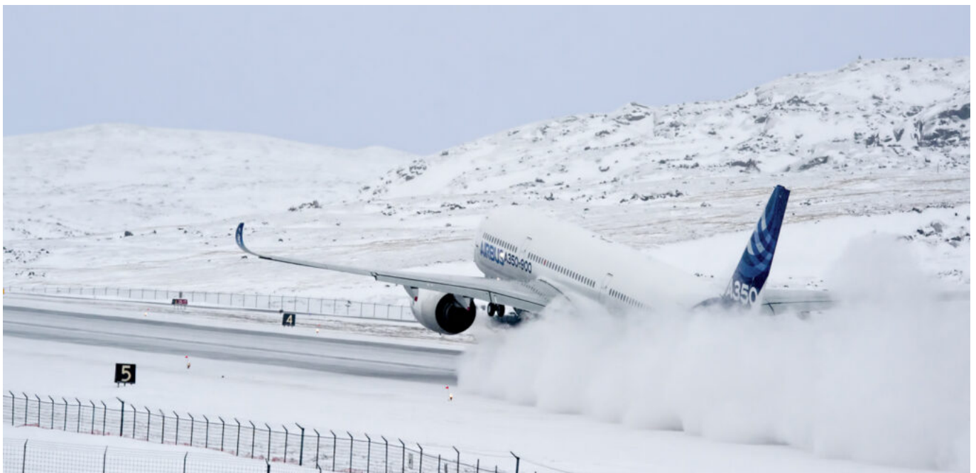
A350 contaminated runway tests (credit: Airbus).
