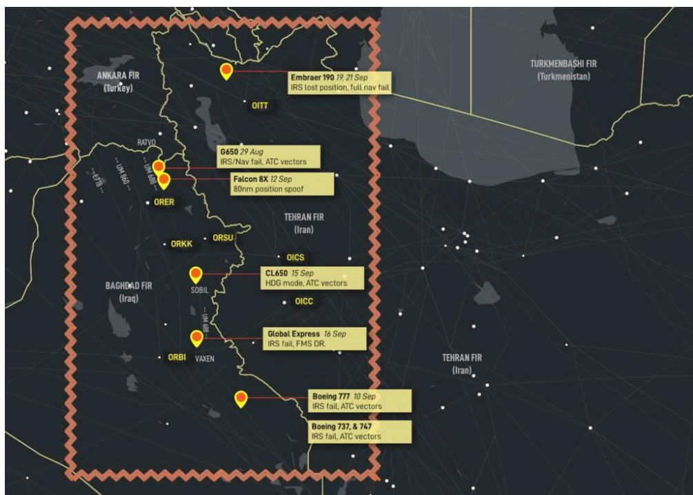
The **Baghdad** spoofing type involves GPS spoofing of enroute aircraft, nav failures follow. This was the first type of spoofing, initially reported on August 29, 2023, with a large amount of further reports starting in September 2023.
