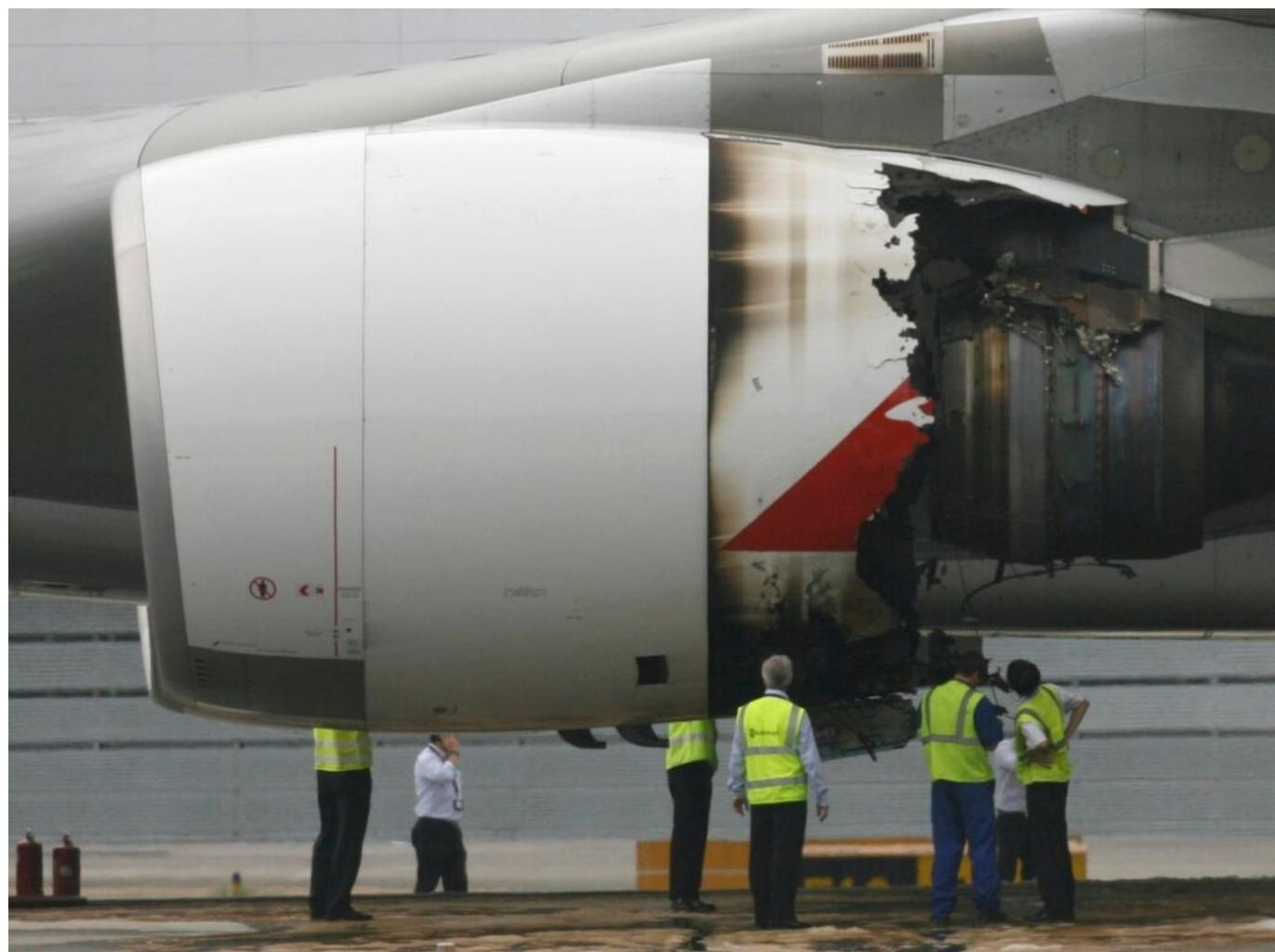
After a single engine failure the crew of QF32 were faced with 43 different failure messages in the first sixty seconds.
