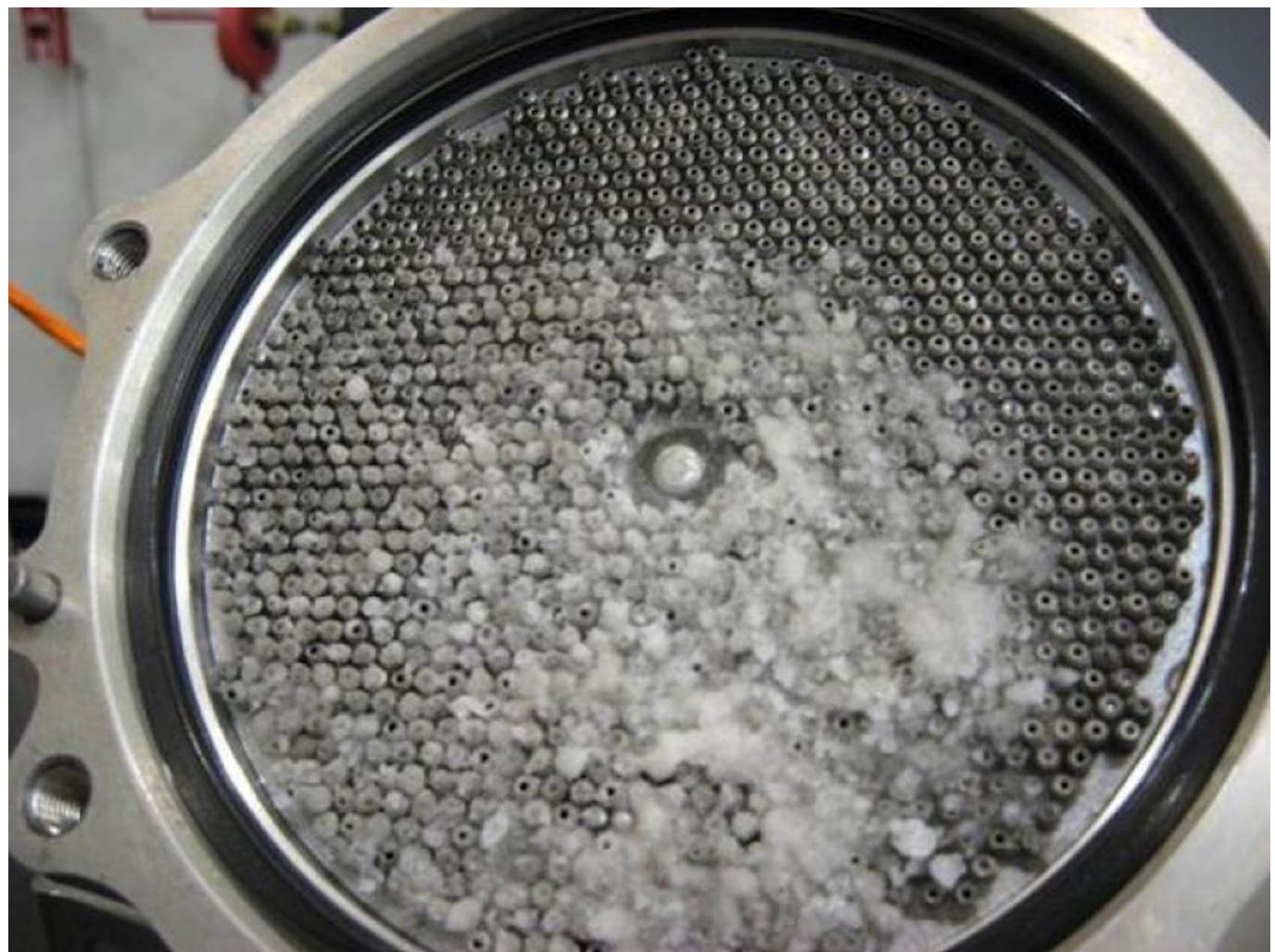
Icing can clog filters and prevent fuel from reaching your engines.
