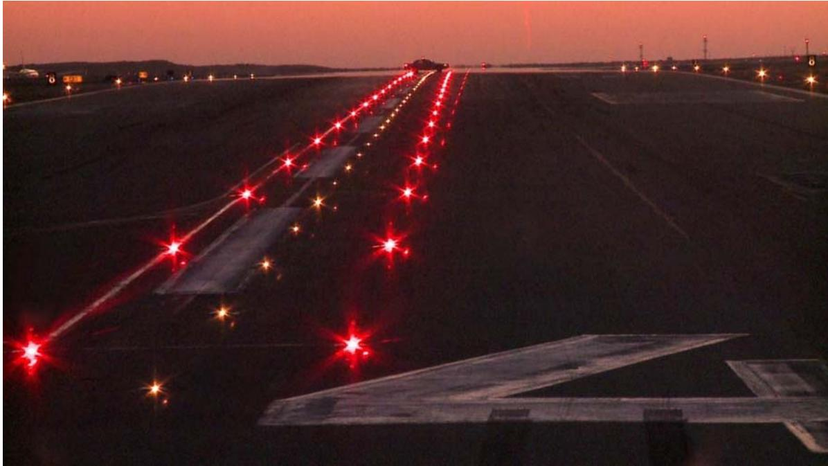
As you may know, the FAA is working on Runway Status Lights (RWLS). It's a new system that's live at 20 airports in the US. Basically, you get a nice set of red lights (embedded in the ramp) that tell you whether it's safe or not to proceed. These lights are installed (or placed or located) at the entrance of the runway and at the start of takeoff. If any of these lights are red, you don't go. Simple as that.
