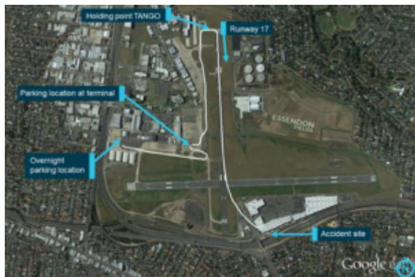
The pilot at the controls of a Beechcraft B200 Super King Air that crashed shortly after take off had the aircraft's rudder trim in the full left position for take off, the Australian Transport Safety Bureau (ATSB) has found.
