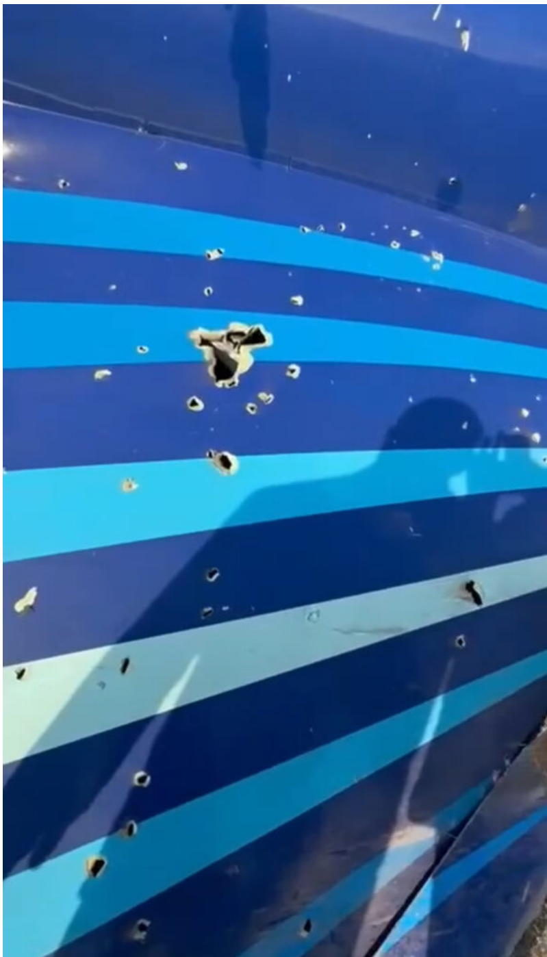
Photos of AZ8243 seems consistent with shrapnel damage likely
