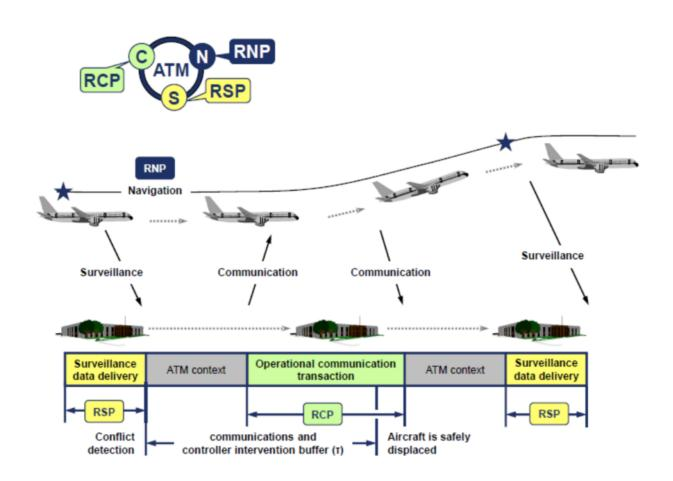
So, we have a loop here, **C-N-S. Communication**, **Navigation** and **Surveillance**. An aircraft sends surveillance information to ATC about where it is; the aircraft stays within confines of RNP navigation requirements and ATC communicates with the aircraft within the required transaction times. *Pretty easy!*
