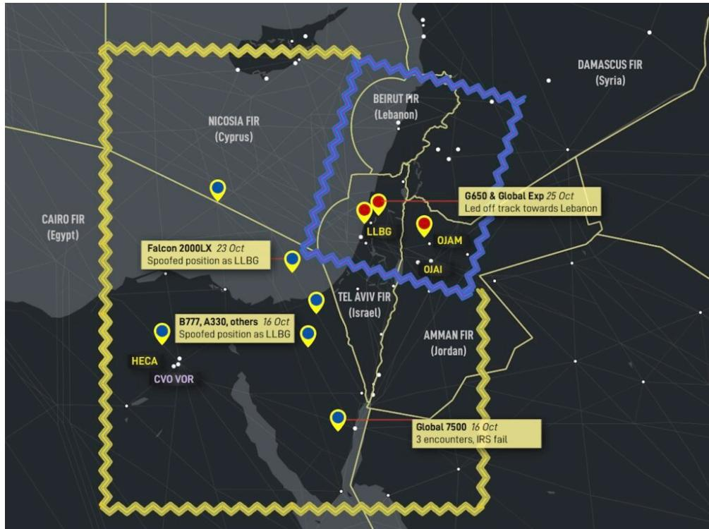
These reports first surfaced around Oct 16. Most reports are within the Cairo FIR. All crew reported similar circumstances, where a false or spoofed GPS position is received by the aircraft, incorrectly showing the aircraft position as being over LLBG/Tel Aviv. Locations vary from airways over the eastern Mediterranean, Egypt, and also on approach into Amman, Jordan (OJAM). Reports range from 100nm to as far as 212nm from LLBG.
