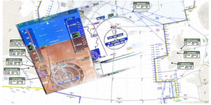
An increasing issue for the NAT Oceanic FIR's is how to handle aircraft with an in-flight degradation of GPS. This normally follows a **GPS Spoofing encounter** somewhere prior to Oceanic Entry, leading to a degraded RNP capability.
