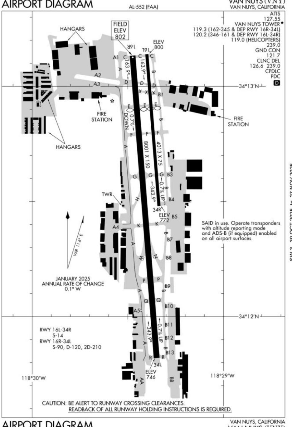
Based on the Notams available right now, **the short runway 16L/34R has no closures planned**. But watch out here – it's only 4000ft long, is limited to a single wheel configuration with a max weight of about 14000 lbs, so it will not be an option for most BizAv aircraft during the closures.
