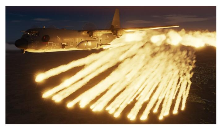
Magnesium flares burn extremely hot and cannot be put out with water or halon. Which is why accidental activations are a major concern on the ground, and aboard the aircraft.
