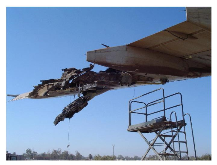
Aircraft are most at risk from MANPAD attack during take off and landing – like this A300 which took heavy damage to its wing departing Baghdad airport.
