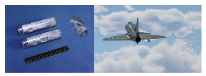
Chaff systems spread a cloud of small, thin pieces of radar reflective material.
