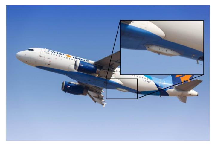
The recent application to the FAA was to install infrared pods like this one. The problem for the industry is cost.
