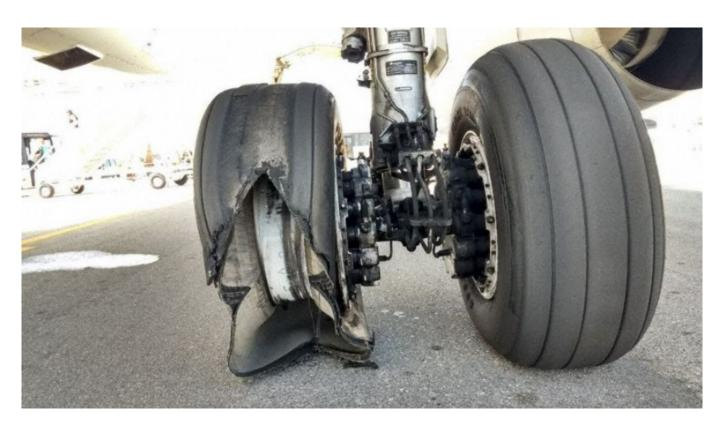
Tire failure - one of the leading causes of high speed RTOs
