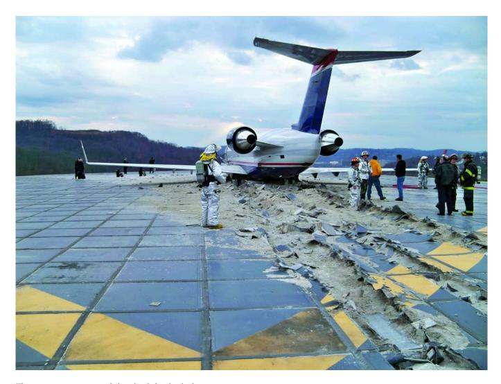
The arrestor system doing its job nicely here
