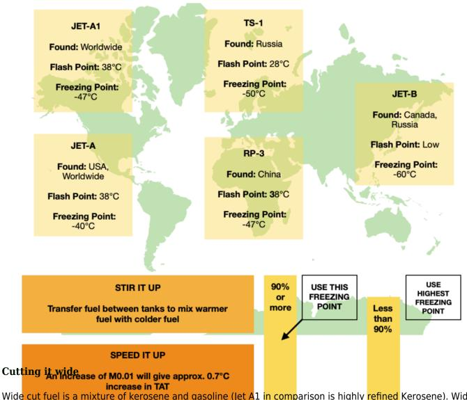
Wide cut fuel is a mixture of kerosene and gasoline (Jet A1 in comparison is highly refined Kerosene). Wide cuts are not often recommended by airplane manufacturers because the quality and performance specifications are generally got assigned.
