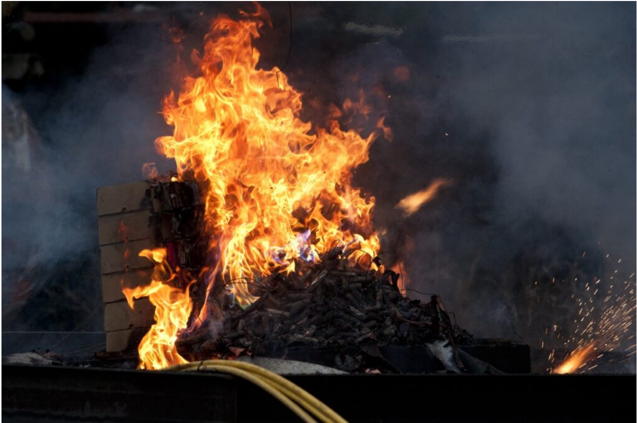
An FAA fire test with 5000 lithium ion cells
