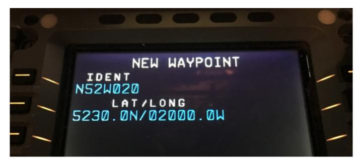
The ident doesn't show the half waypoint – so the full waypoint must be checkedStill confused about what to insert? Read this handy guide from Honeywell.
