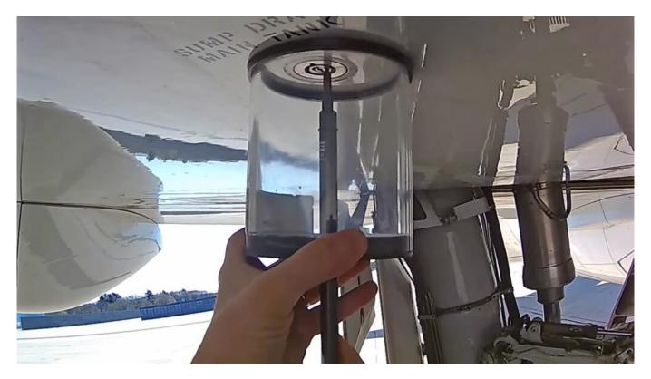
It is becoming mandatory to test fuel samples both before and after refuelling.
