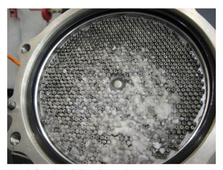
Icing can clog filters and prevent fuel from reaching your engines.
