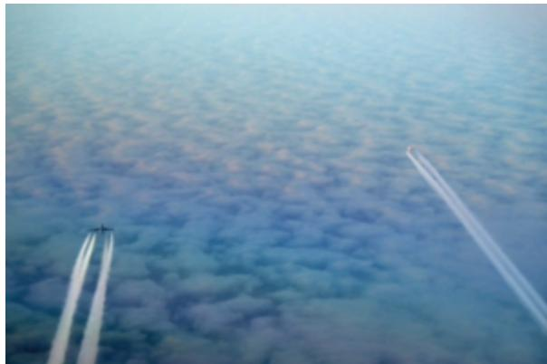
GPS technology allows modern jets to fly very accurately, too accurately it turns out sometimes! Aircraft can now essentially fly EXACTLY over an airway/track laterally (think less than 0.05NM), separated only by 1000FT vertically. A risk mitigation strategy was proposed over non-radar airspace to allow pilots to fly 1-2 nautical miles laterally offset from their track, **randomly**, to increase flight safety in case of any vertical separation breakdown.
