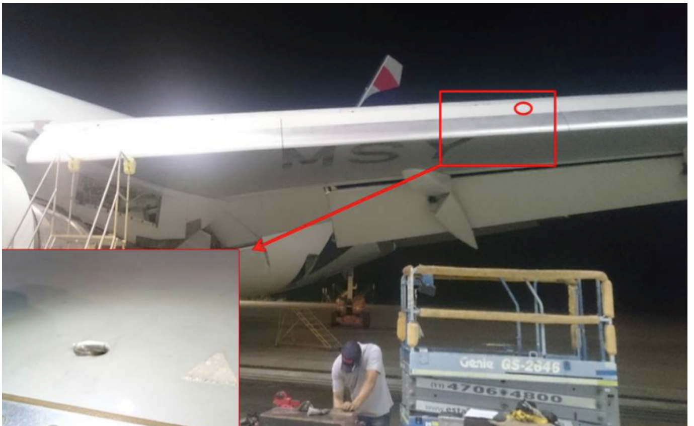
Section of wing with lodged bullet
