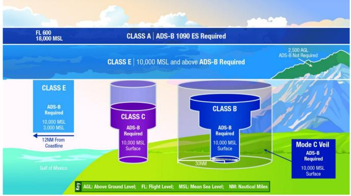
Also, according to the US AIM, operators flying at 18,000 feet and above will require equipment which uses 1090 ES (extended squitter). Those that do not fly above 18,000 may use either UAT (Universal Access Transceiver) or 1090ES equipment. For international operations 1090ES is by far the most accepted system.
