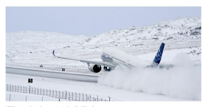
A350 contaminated runway tests (credit: Airbus).
